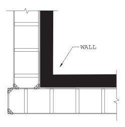
Second, when adjacent intersections occur within a space too narrow to allow corner brackets to be inserted between the intersections. Minimum space requirements are given below.
