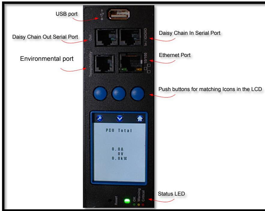
You can link (daisy chain) up to 20 PDUs together (1 Primary and 19 Secondary) and access all of the PDUs from a single Ethernet network connection to the Primary PDU.
