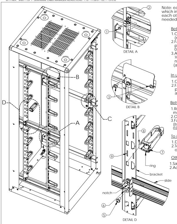
Note: each bracket has one NOTCHED END. Regardless of which installation style you choose, the notched ends must face each other as shown in Detail D. More hardware is supplied than needed for some installation styles.
