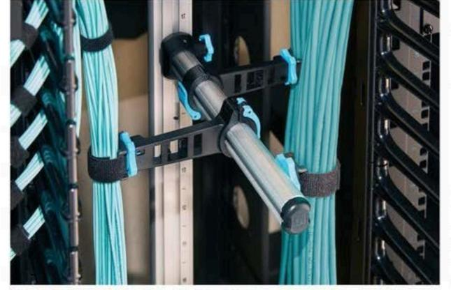
Advanced, high-wattage technologies require properly spaced, smaller cable bundles to avoid excessive heat accumulation. Cable managers with a central track system allow cable bundles to be properly spaced and fully supported precisely where needed.
