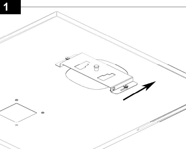
Place the components on a flat work surface. Loosen the thumb nuts 1-2 turns, but do not completely remove. Slide the mounting bracket in the direction indicated.
