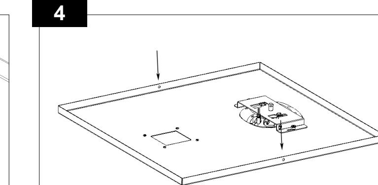
Remove the ceiling tile where the mount is to be placed and place the panel into the ceiling grid. Put the ends of the Caddy Speed Link™ support through the holes in the side of the mount and attach the free end to a structural element in the ceiling.
