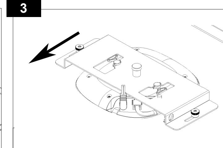
Align the mounting feet on the AP with the slots in the mounting bracket and slide the bracket in the direction shown until the plunger depresses into the AP. Tighten the thumb nuts to secure the mounting bracket. Additionally, a lock may be inserted through the mounting plate and hasp to secure the AP.
