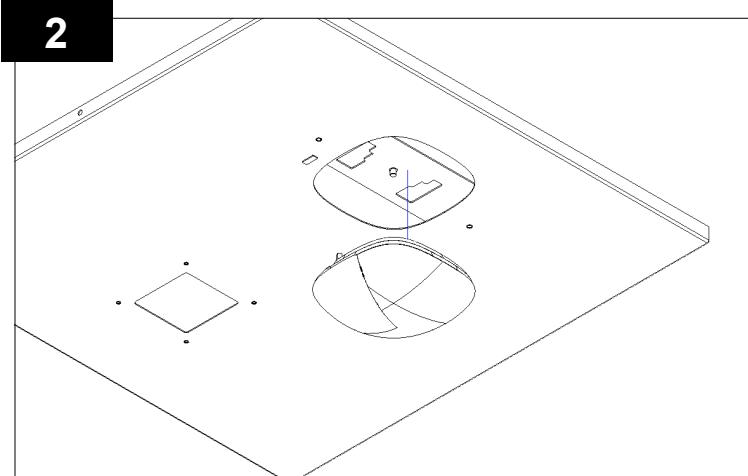
Insert the Aruba AP from the bottom side of the mount.
