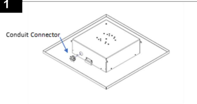
Find a flat work surface to assemble the ceiling enclosure, access point, and antenna(s) prior to mounting in ceiling.
