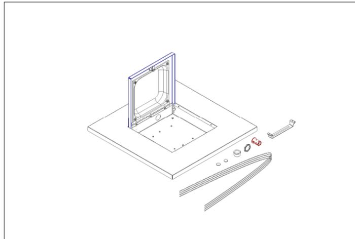
The locking Model 1052-CP and 1052-DOME series enclosures provide a convenient way to mount and secure APs in a suspended ceiling. The AP is mounted in the backbox. Interchangeable retrofit doors permit vendor and technology migrations, and simplify moves, adds, and changes. UL listed for installation in the plenum space.
