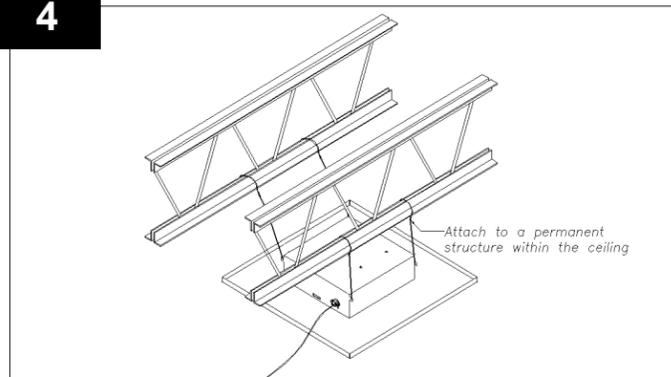
Use minimum 12-gauge support wire (included) to support the access point enclosure independently of the ceiling grid. Attach one end of the wire to the support wire tabs located along the edge of the back box and the other end to a permanent supporting structure within the ceiling such as a ceiling joist.
