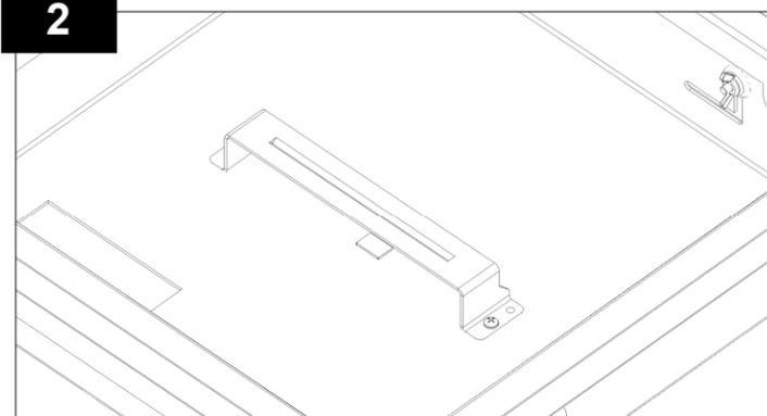
Install the provided T-bar mount into the enclosure.
