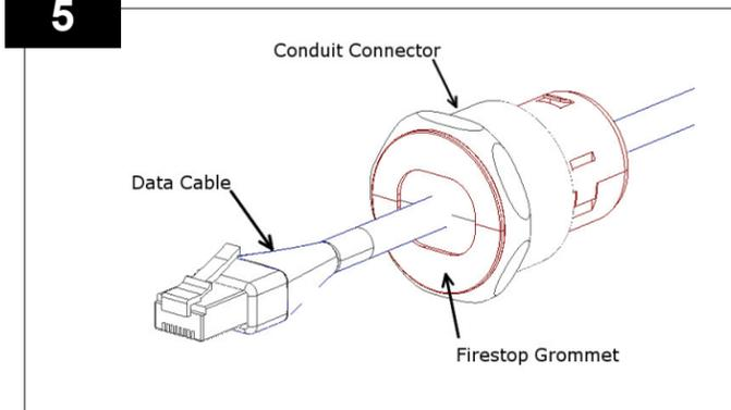
Run the data cable through the conduit connectors located on sides of the enclosure backbox. Pull the data cable through the conduit connector far enough to allow attachment to the access point (8" - 10"). Snap the firestop grommet on to the cable and slide it inside the conduit connector.
