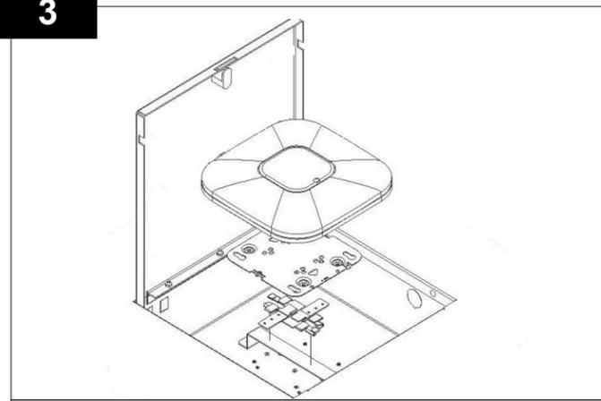
Use the manufacturer's T-bar mount clip to attach the AP to the T-bar mount. Additional components may be required from the AP manufacturer.
