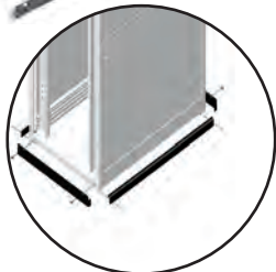
Seal Kit Installation
