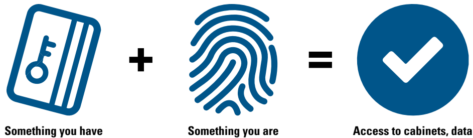
Figure 3: Locks with multifactor capabilities combine multiple key types to enhance security and connect credentials to specific authorized users.
