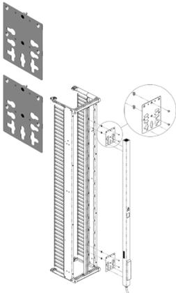
**Dual PDU Bracket Kit for Motive Vertical Cable Manager**
