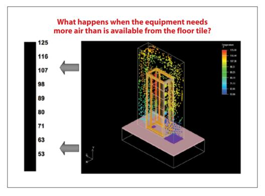
ple use a specific brand of cabinet that has the patented ability to deliver cold air to the top of the cabinet using side air ducts installed within the cabinets. This is a relatively new and inexpensive way of getting cold air to the top of the cabinet and it does not add any extra moving parts that can break down or use any more electricity.
