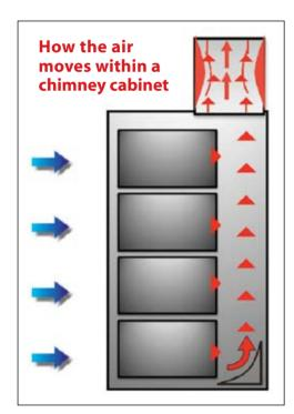
I recommend using a hot air return chimney on each cabinet that can be ducted straight back into a ceiling return plenum or can take the hot air away from the cabinet and direct it to the top of the room where it makes its way back to the CRAC units without mixing with the supply air. This means that each cabinet is its own segregated island with cold air being delivered to the front of the cabinet through a perforated door and hot air being sent out the top of the cabinet.
