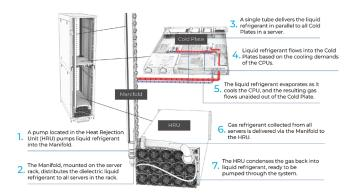
Engineered refrigerant dielectric fluids are designed to evaporate at much lower temperatures than water, allowing liquids to transform into vapor and then condense back into liquid form at temperatures that are much lower than the boiling point of water. Heat can be rapidly transferred away from the equipment, allowing for improved cooling performance and maintaining lower operating temperatures.
