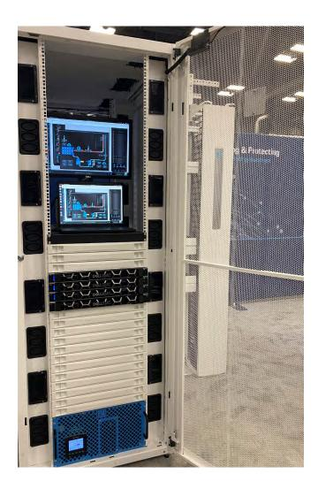
rack with the integrated liquid cooling system when used in conjunction with a shock pallet. Equipped with in-rack eConnect® power distribution units (PDUs), Chatsworth's cabinets provide a complete solution to power and manage high-density loads, close to the device. The cabinet design and size allow liquid cooling to be added while preserving the ability to meet cable management standards.
