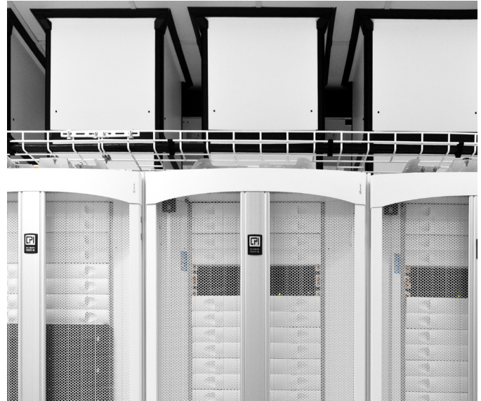
CPI's Vertical Exhaust Ducts guide hot exhaust air from the back of the cabinet to the drop ceiling plenum, creating a closed hot air return path to the cooling system.
