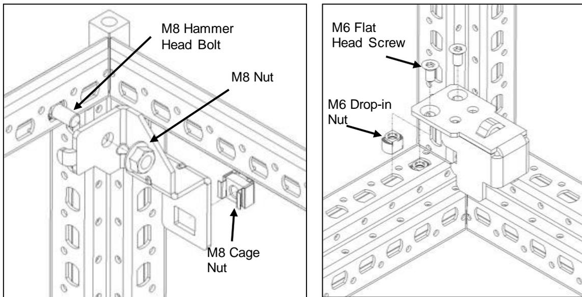
4. Move the top and bottom brackets to the desired frame depth location. To remove the threaded bolts or drop-in nuts from the frame, rotate each 90 degrees to extract from hole. To install brackets at new location, rotate the threaded bolts or drop-in nuts 90 degrees to engage frame.
