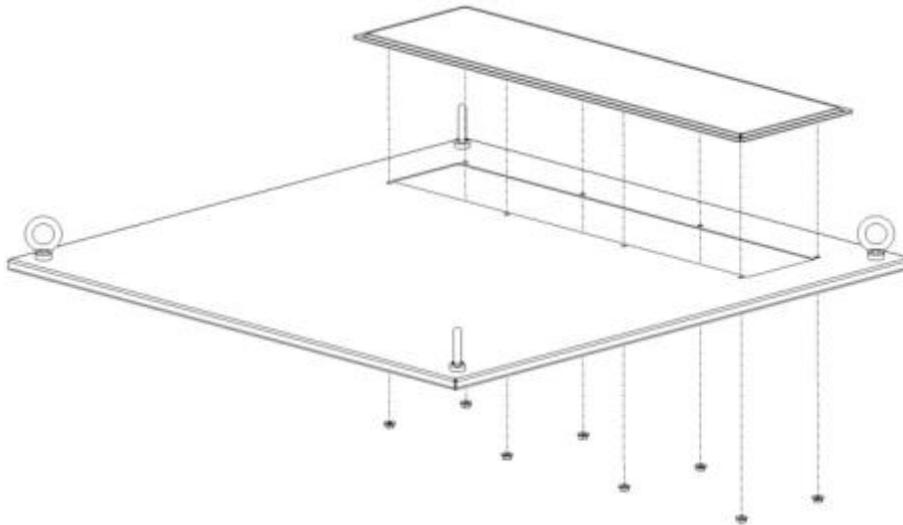
1. Use a 10mm socket wrench to remove or install the gland plate for the top panel if included.
