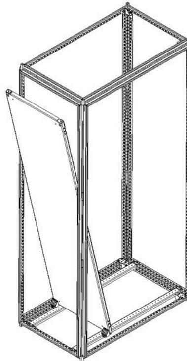
1. Verify the bottom support rails are installed. Do not remove (or install) the mounting panel without the support rails being installed.
