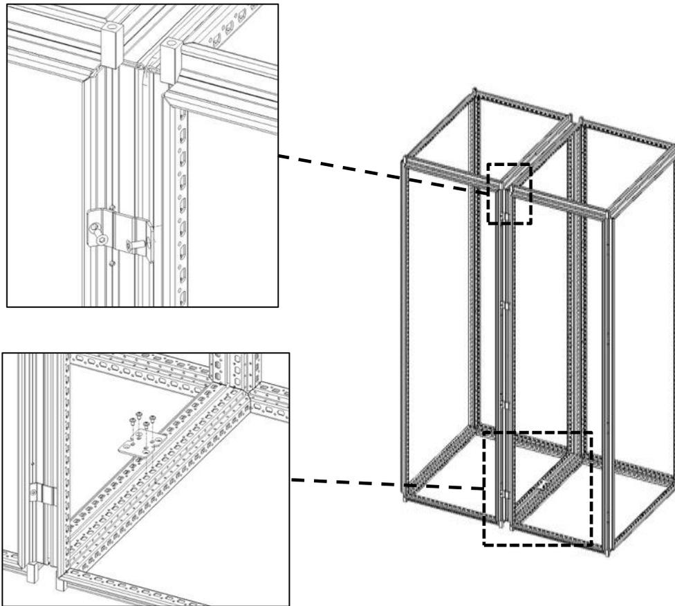
3. Move the second cabinet so that the cabinets are aligned. This may also require adjusting the leveling feet if the second cabinet was not set at the same level as the first cabinet.
