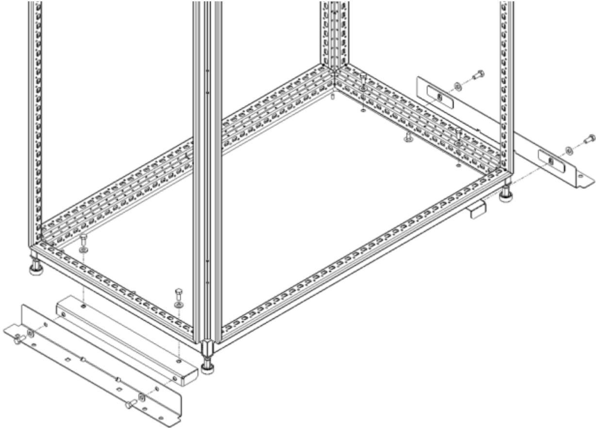
Attach the cabinet to the floor with 3/8" or M10 hardware appropriate for your type of flooring.
