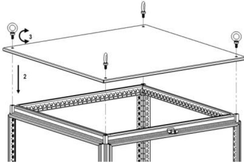
3. Install the four eyebolts to attach the top panel to the cabinet frame.
