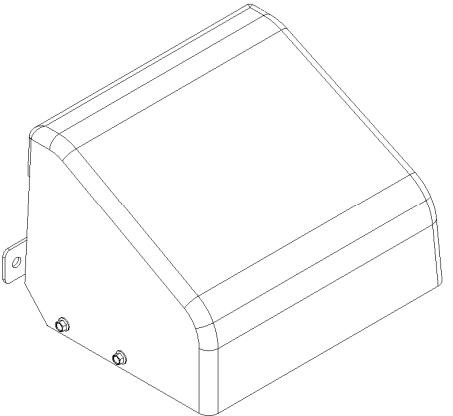
This compact cover is designed specifically to conceal and protect outdoor rated APs in challenging environments such as stadiums, auditoriums, and gymnasiums. The ABS cover can protect the AP from impacts. The cover is also paintable and transparent to wireless signals. As a result, APs with body integrated antennas may be protected. Compatible with Cisco AP 1532i and 1562i and Aruba AP-277, AP-377, and AP-577. The 3009 is ideal for under-seating installation.
