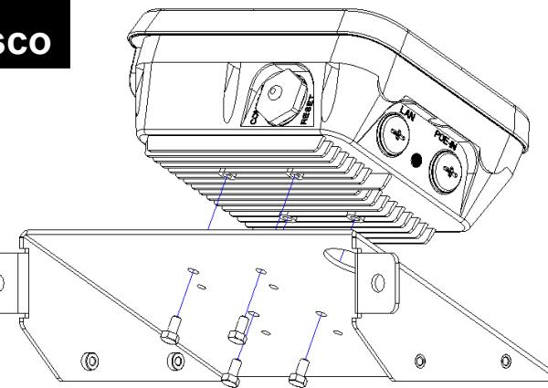
For installations with a Cisco AP 1532i or 1562i, detach the AP bracket included with the Cisco AP. Remove the four (4) hex head screws from the back of the AP. Retain the screws.
