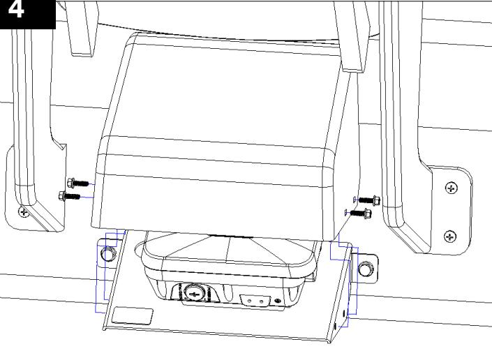
Place the cover on the base then secure it with the four (4) 1/4"-20 flanged hex head screws that were removed in step 1.
