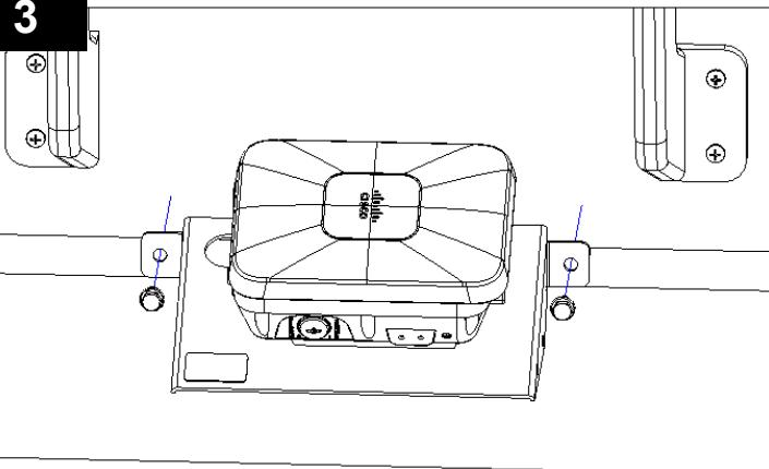
Fasten the base down with appropriate hardware (not included) to studs or masonry.
