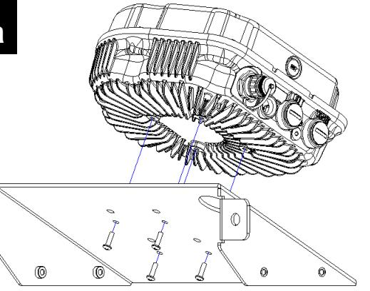
For installations with a Aruba AP-277, AP-377, or AP-577, detach the AP mount included with the Aruba AP. Remove the four (4) pan head screws from the back of the AP. Retain the screws.
