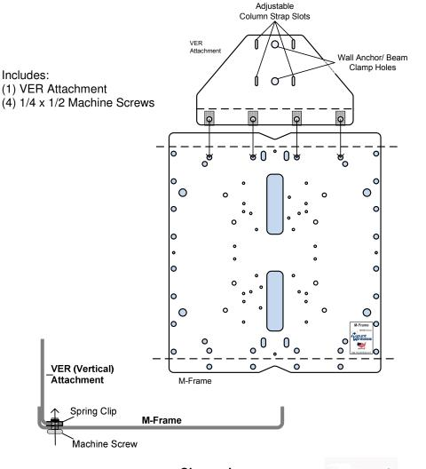
Column Strap Slots VER Ω Attachme Wall Anchor/ Beam Clamp Holes Includes:  $\cap$ (1) VER Attachment (4) 1/4 x 1/2 Machine Screws 0 ¥ 0 ۰ 0 0 0 0 o 0 o 0 0  $\circ$ 0 0 M-Frame Lount 0 0 0 -0 0 0 0 0 0 VER (Vertical) 0 0 Attachment M-Frame Spring Clip **M-Frame** Machine Screw Oberon, Inc State College, PA ●):::=:(O)î 814-867-2312
