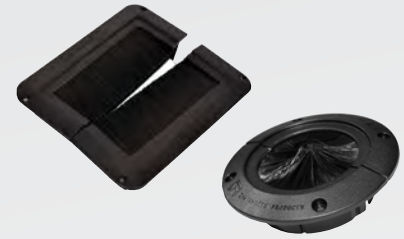
Figure 5: Raised Floor Grommets are available in various sizes and shapes. They seal openings in raised floor tiles with brushes or rubberized gaskets to reduce air leaks around cables, conduit and piping. Use these grommets to seal openings in raised floor tiles when the interstitial space under the floor is used as a supply air plenum.
