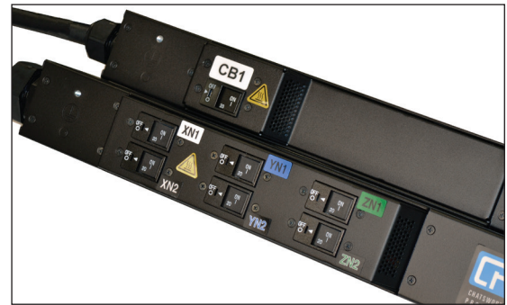
Low-profile, UL 489 listed, magnetic-hydraulic breakers handle higher temperatures, prevent nuisance tripping and do not block airflow through the cabinet.
